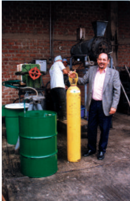
Storing oil in 200 l barrels, in an inert atmosphere, prior to export. Lima, Peru. Photo D. Pioch.
