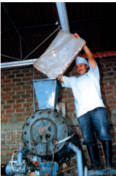
Loading a preheating module prior to a continuous oil pressing operation. Lima, Peru. Photo D. Pioch.
