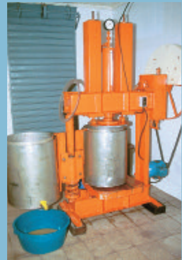
Oil production. Handmade hydraulic press (batch pressing). Laranjal do Jari, Brazil. Photo D. Pioch.
